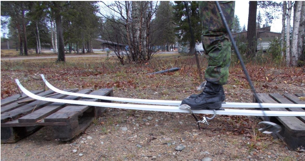
Pending/sag, simulated ditch crossing.
