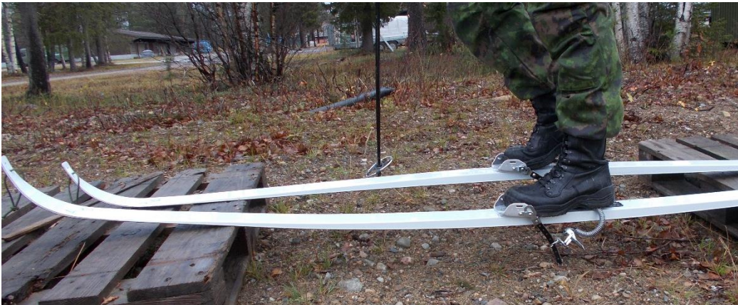
Pending/sag, simulated ditch crossing, weight on one foot only.
